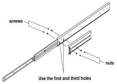
Attach the rear mounting brackets to the back side of each slide using two 8-32 x 3/8 pan-slotted phillips screws and two 8-32 keps nuts. Do not tighten the screws.
